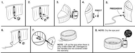
Make sure the spa and pump are completely dry. This is essential to extend the life of the spa. We recommend using the pump to blow dry the spa, pump and pipes. Remove the filter sets and discard the used filter cartridges. Re-attach the two stopper caps onto the spa's inlet and outlet valves. It is recommended you store the spa in its original package in a warm [above 15°C (59°F)] and dry place.
