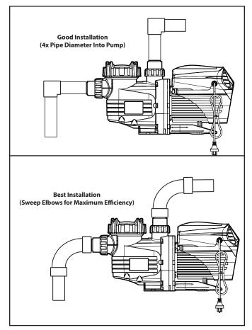
Figure 6. Viron XT Series 2 Pump Good Piping Installations
