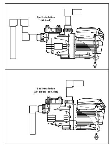
Figure 5. Viron XT Series 2 Pump Incorrect Piping Installations
