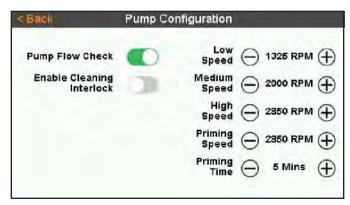
Figure 25. Pump Configuration
