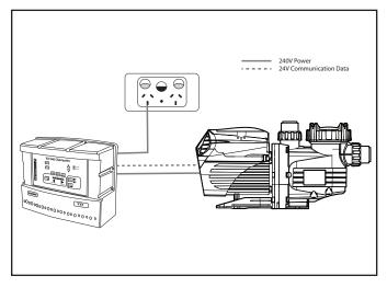
Figure 27. Viron XT Series 2 Pump, Compatible VX Timer Model Chlorinator and Remote Control
