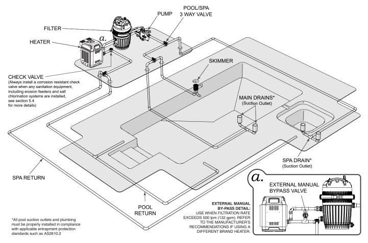
Figure 8. Typical Water Piping Configuration
