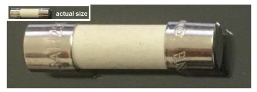
Fuse size is M205 (20mm x 5mm), TD6.5A (TD – Time Delay / slow-blow), HRC (High Rupture Capacity).
