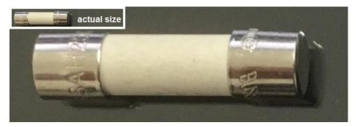
Fuse size is M205 (20mm x 5mm), TD5A or TD6.5A (TD – Time Delay / slow-blow), HRC (High Rupture Capacity).
