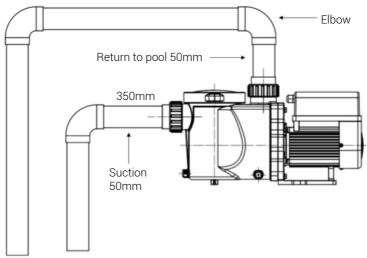
\* The pump inlet/ outlet union size: optional with metric 50 or 40mm.
