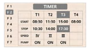
Insnrg will send the Variable Speed Pump factory programmed with start time of 08:00 and stop 12:00 for Timer 1, then 18:00 start and 20:00 stop for Timer 2. If you are happy with this, you can leave as factory settings. To change the timer settings, select the Timer Period you wash to adjust by pressing the corresponding button below the screen. Similar to the Clock
