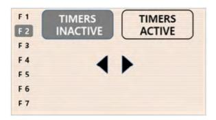
If "Timers Active" selected, screen will then displays timer 1 (T1) to Timer 4 (T4) above 4 horizontal buttons beneath LCD screen and a summary of timer periods as below.
