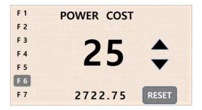
Press up or down to change from 5 to 40 in 1 cent increments. This value represents cents per kW hour and can be located on your latest electricity bill to get the most accurate results.
