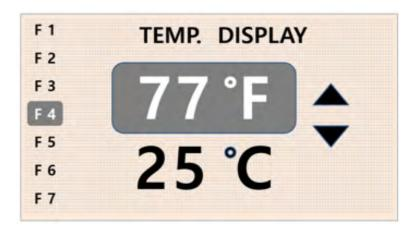
Press up or down to select your preferred display in either "C" (Celcuis) or "F" (Fahrenheit). If no external temperature sensor is fitted to your Pump the display will show "0" values, contact your pool professional to confirm if this is correct.
