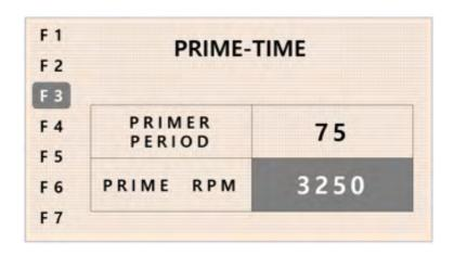
When "on" is selected "primer period = mmm: XXX". Press up or down to select from "0" to "120" minutes. Scroll right or left to select Prime RPM, press up or down to select 1200 to 3300 in 25 RPM increments.
