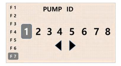
A Pump ID may be required when using an Automated system that requires a Pump to have an ID to ensure it operates in the correct time and speed. Your pump will default to Pump ID 1, should you need to adjust, scroll left or right to appropriate number, then press up or down to select. Choices are 1, 2, 3, 4, 5, 6, 7, 8.
