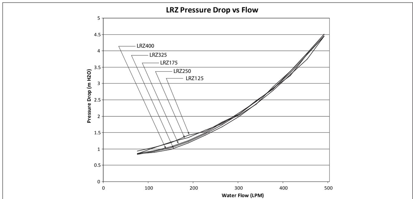
Figure 7. Hydraulic Head Loss Curve
