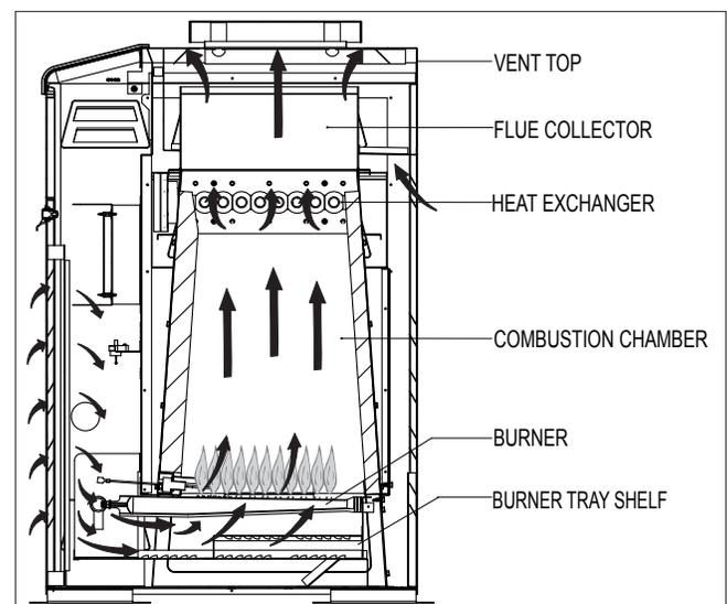
Figure 23. Atmospheric Combustion System
