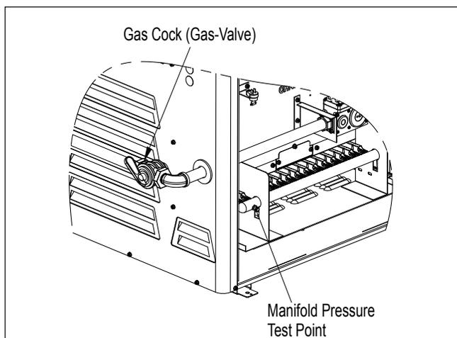
**Figure 5. Fitting a Gas cock (gas-valve)**
