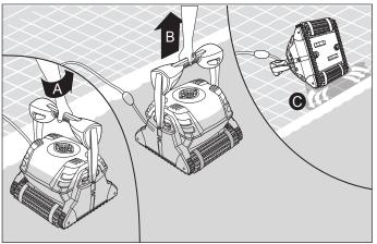
Using the floating cable, bring the Pool Cleaner to the pool's edge.
