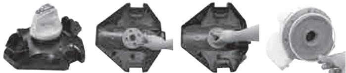
2. Use the screwdriver to unscrew the 4 screws located on the bottom of the head to release the bottom plate at first. Use the screwdriver to unscrew all the screws on the base as shown. Remove the impeller and then pry up the base and remove it to expose head inside.
