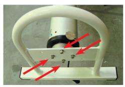
**6.** Install the end frame, secure firmly 4 x mounting bolts
