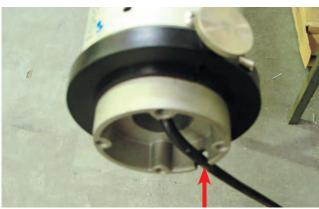
**5.** Ensure drive motor wire is running through the recess in the housing on the end
