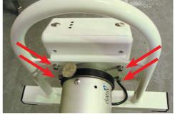
**7.** Install the control housing, secure firmly the 4 x mounting bolts
