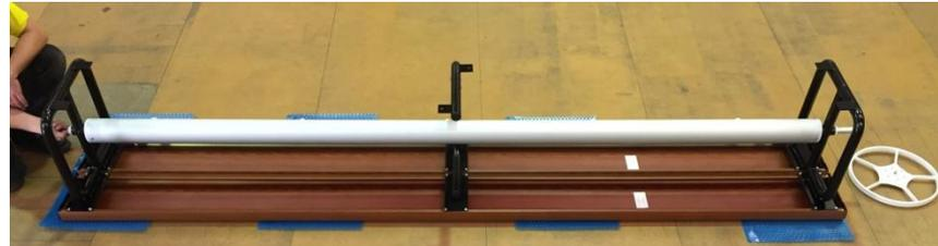
7. Install the hand wheel adaptor on the drive end of the roller tube
