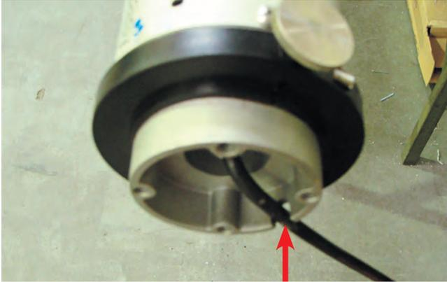
**5.** Ensure drive motor wire is running through the recess in the housing on the end
