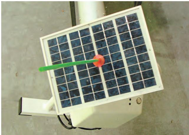
10. Adjust the solar panel position by placing the shadow indicator in the centre of the solar panel, at midday adjust the position of the solar panel so there is minimal shade from the indicator. This will ensure the optimum solar panel position for your location
