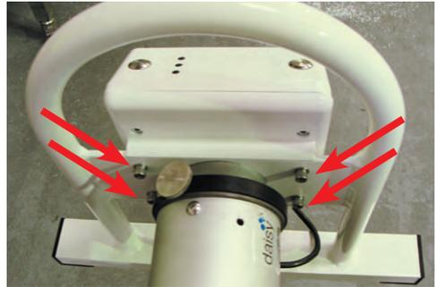
**7.** Install the control housing, secure firmly the 4 x mounting bolts
