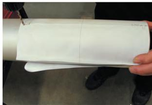
**2.** Without the drive motor inside the tube, mark and drill the 6 x 4.5mm holes through the template with the 4.5mm drill bit (3 around the end of the tube and 3 around the inside of the tube approximately 243mm from end of tube)
