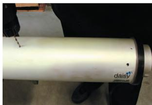
**3.** Insert the drive motor, (if there is a feather plug in way, remove, then replace after motor install) then using the 4.5mm drill again, drill through the 6 holes in the tube, through the drive motor flange
