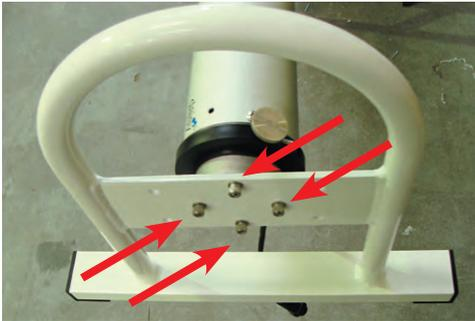
**6.** Install the end frame, secure firmly 4 x mounting bolts
