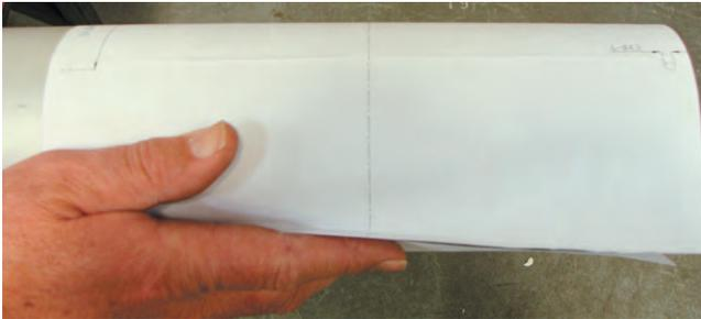
**1.** Wrap paper template around roller tube, the end you want to install the Daisy Power motor and controls
