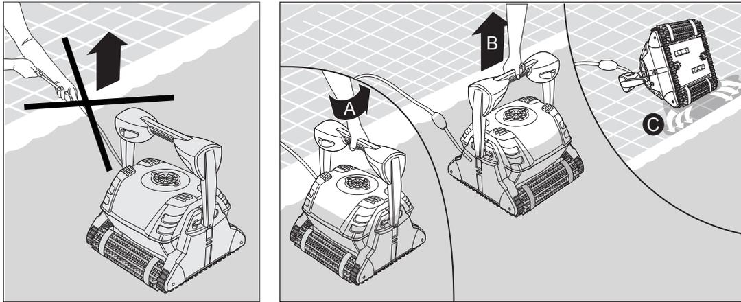
Using the floating cable, bring the Pool Cleaner to the pool's edge.
