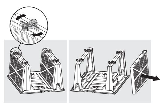
Open the clips and remove the filters.
