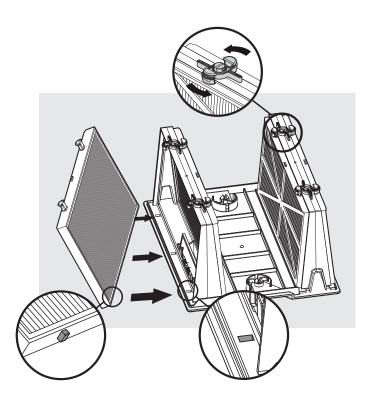
Insert the filters with the plastic backing facing out. Insert the cartridge unit.
