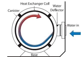
✓ The titanium **dual coil** heat exchanger is highly resistant to ozone, iodine, baquacil, salt and chlorinated water
