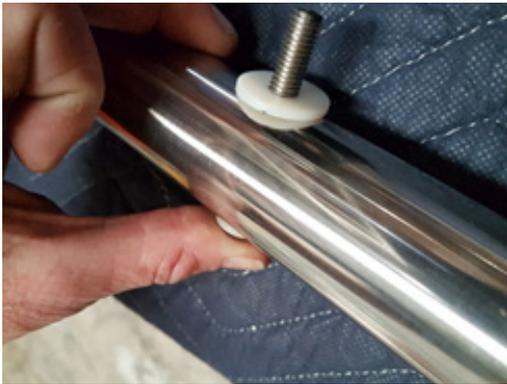
2- Starting with either the top step or bottom step, insert the M8 x 60 through both holes on one of the ladder rails, then fit a Large Nylon Washer on the inside of the ladder rail
