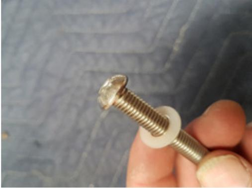
1- Fit 1x Small Nylon Washer onto 1x M8 x 60 Button Head (do this for both screws)
