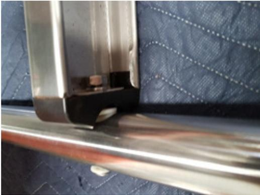
4- Fit a spring washer then a M8 hex nut to the M8 x 60.
