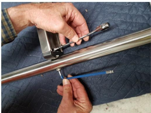
7- Using your allen key & spanner, tighten the hardware.
