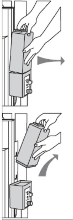
**To remove** - pull the battery pack away from the mounting plate so that the latch on the battery pack clears the side tabs on the mounting plate - then lift the battery pack up and away from the Control Box.
