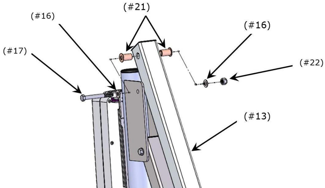
14. Attach the opposite ends of the Actuator Arm Assembly (#12) and Support Arm Assembly (#13) to Seat Bracket with (2) Bolts (#17), (4) Washers (#16) 4) Bushings (#21) and (2) Nuts (#22) in appropriate holes of the Seat Bracket (as shown below), following the same sequence as in previous step.
