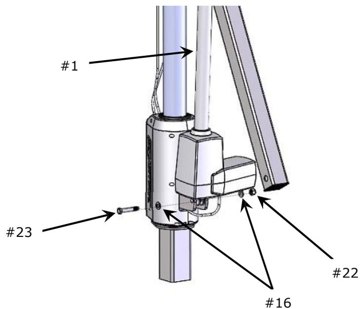
11. Attach the opposite end of the Actuator (#1) to the Actuator Arm Assembly (#12) using (1) Bolt (#23), (2) Washers (#16) and (1) Nut (#22) through the holes in the flanges of the Actuator Arm (see image below).
