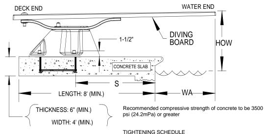
SECURE ALL FASTENERS AND TIGHTEN UNTIL LOCK WASHERS ARE FULLY COMPRESSED
