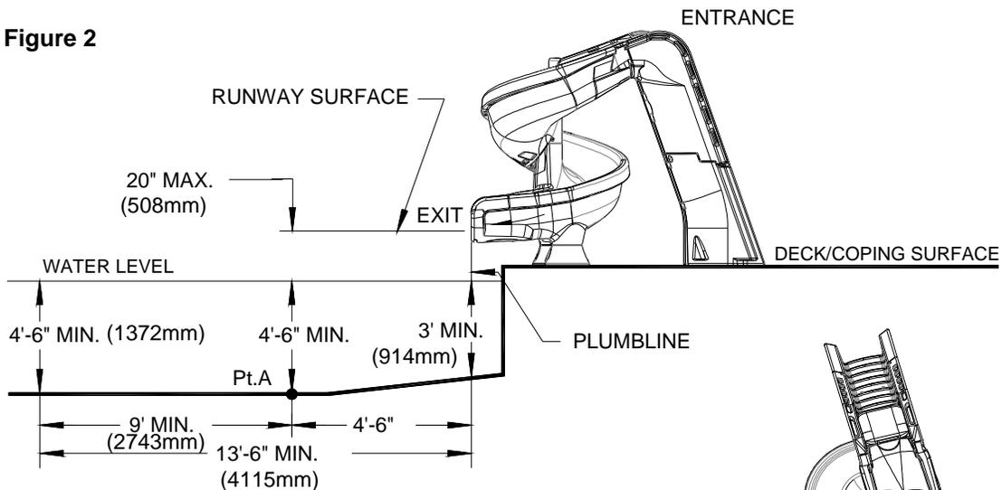
Dimensions are in feet/inches and (millimeters)
