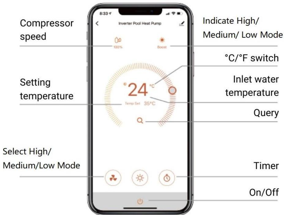
2. For Heat Pump with Heating and Cooling Function:
