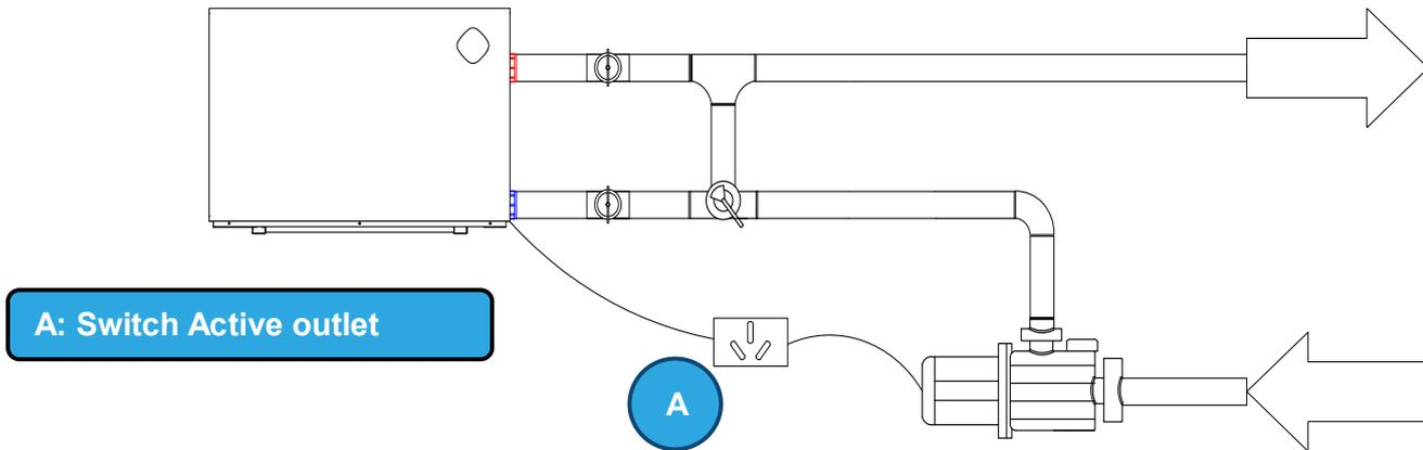
1. Termination points are labelled P1-P2 from the on-board relay and is activated by the timers and pool temperature, and will continue to run the pump until the heated water reaches the set temperature or the timer switches off.
