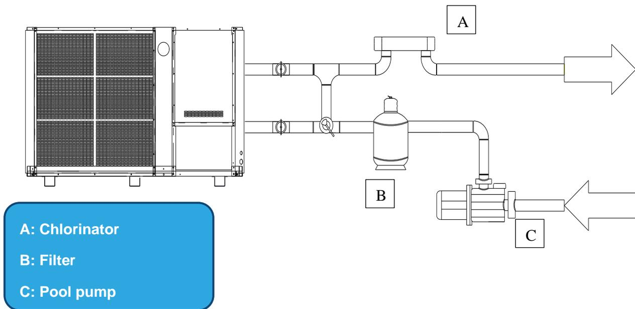
1. Chlorinator controller initiates the filtration pump.
