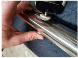
3- Fit one end of a ladder tread over the M8  $\times$  60 ensuring the large nylon washer is in between the rail & the tread end
