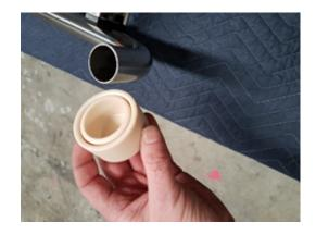
8- If you have ordered a Standard or Flanged Top only Ladder, your Ladder will come with rubber bumpers for the tube ends. These can now be fitted.
