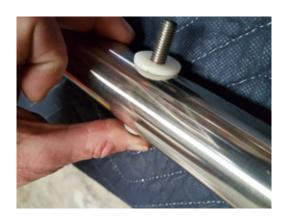
2- Starting with either the top step or bottom step, insert the M8  $\times$  60 through both holes on one of the ladder rails, then fit a Large Nylon Washer on the inside of the ladder rail
