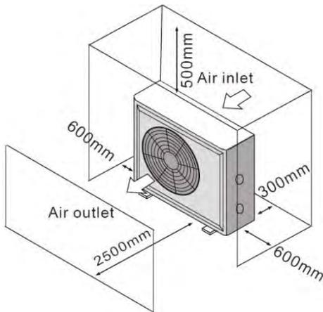
Ensure the heater is installed in a well-ventilated area with plenty of fresh air, a minimum gap between walls/fences etc of 600mm on the sides and 500mm overhead clearance.
