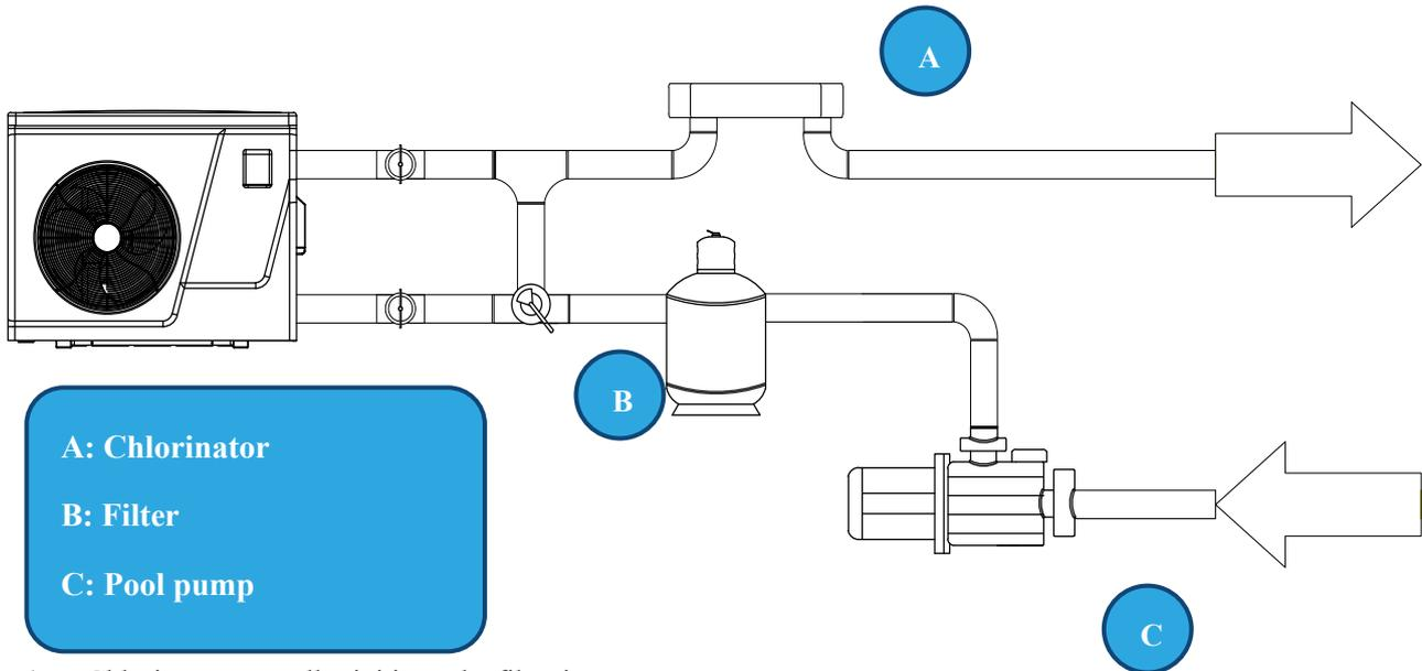
1. Chlorinator controller initiates the filtration pump.
