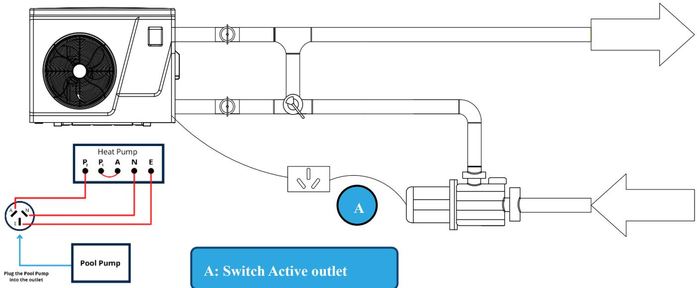
1. Termination points are labelled P1-P2 from the on-board relay and is activated by the timers and pool pump temperature, and will continue to run the pump until the heated water reaches the set temperature or the timer switches off.
