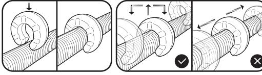
Ideally, the bottom surface of the cleaner should rest flat on the pool bottom. Initially, attach the hose weight onto the first male-female long hose (E) from the hose assembly, close to the next male-female long hose (E). NOTE: Do not try to slide the hose weight along the hose as it could cause damage to itself or the hose. Pull the hose weight upward to detach it from the hose
