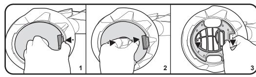
Remove the filter cage and rinse it with clean water. Replace the filter cage if you detect any damage.
