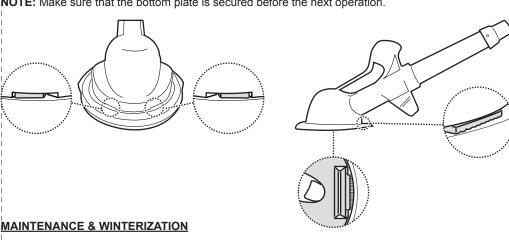
Use clean water to rinse the cleaner, hoses, and other accessories after every use Periodically inspect the cleaner parts and accessories. Replace damaged parts before next use. For winterization, drain the water from the cleaner and accessories. Disconnect hose sections and
