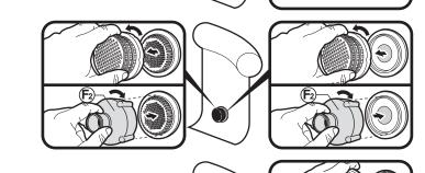
Ø36mm (1<sup>2</sup>/₅in) Strainer hole Remove the grid cover and directly insert the cuff of hose (A) into the strainer hole.
