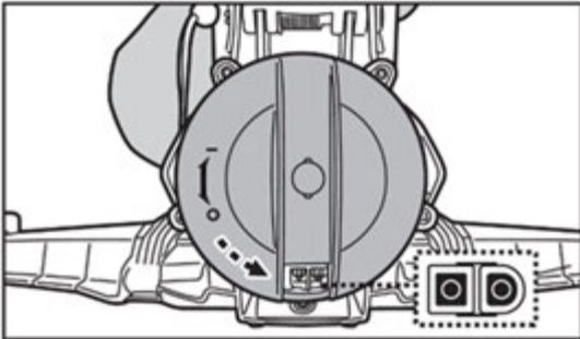
2. Align and attach the charging plug to the charging port. **WARNING!** Be sure not to invert the charging plug and ensure both the charging plug and charging port are clean and dry before charging them. TIPS: Use cotton bud to dry the charging port and pins. Plug the charging cable of the external adaptor into the charging plug.
