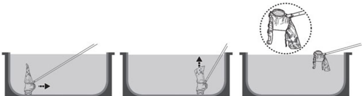
Once the pool vacuum is out of the water, the impeller will cease to spin within 2-3 seconds. The LED light will turn blue. When battery level is running low, blue light will flash.
