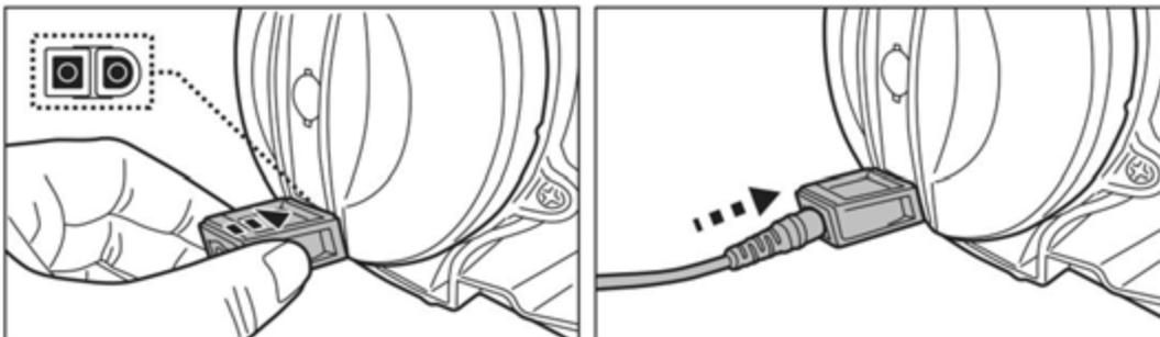
3. Connect the external adaptor to the power source. The indicator light on the external adaptor will turn red when the vacuum is charging and green when it is fully charged. Charge it for 5-6 hours for best performance.
