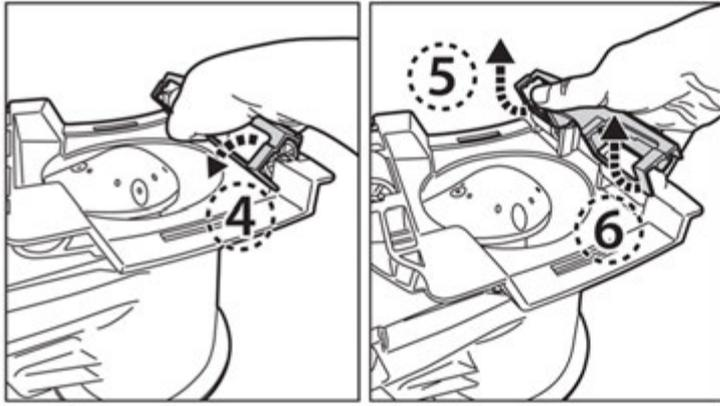
Before detaching the damaged front wheels, you will need to detach the frame first.
