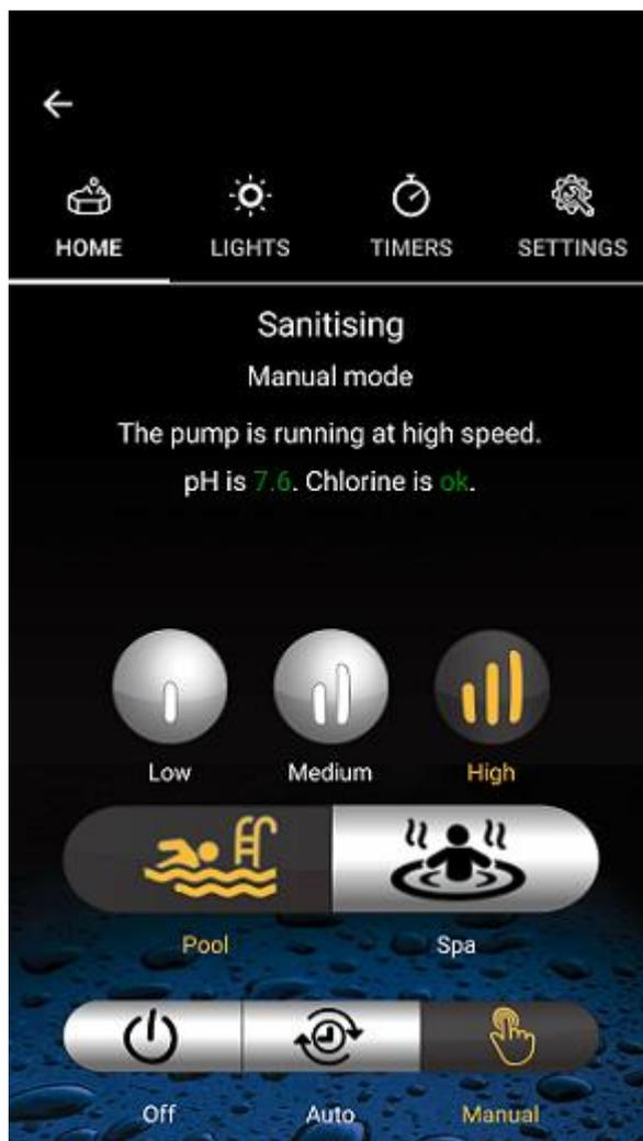
From this page you can turn the Chlorinator On, Off or to Auto, select Pool or Spa Mode and set the pump speed (if a compatible AstralPool pump is installed)
