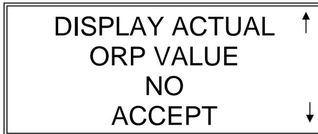
The default value is No, so that during operation the screen will only display "Chlorine OK, Chlorine High or Chlorine Low". Use the arrows up or down to change the default to "YES" and the screen will then display actual ORP levels.
