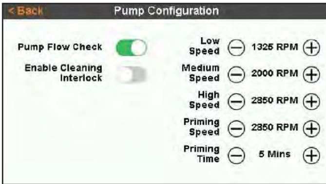
Figure 25. Pump Configuration
