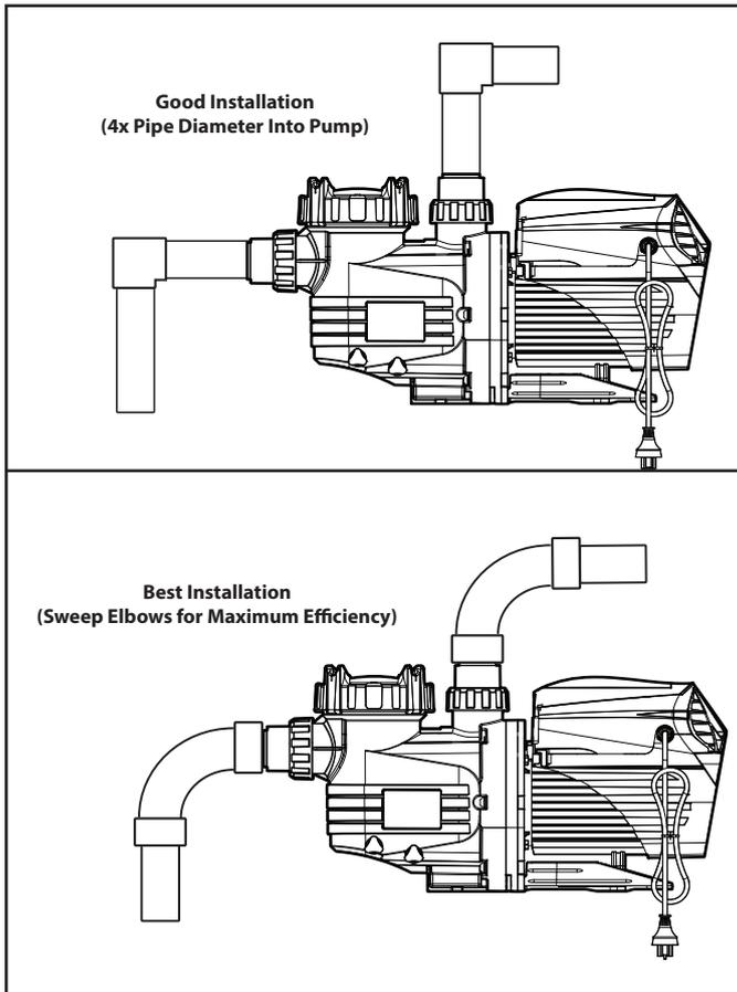
Figure 6. Viron XT Series 2 Pump Good Piping Installations
