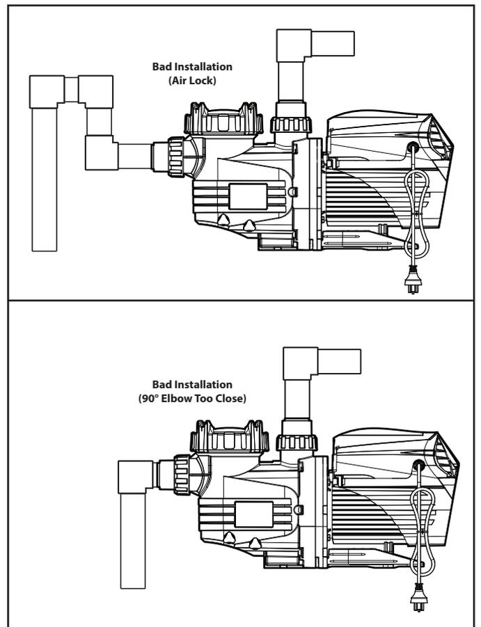
Figure 5. Viron XT Series 2 Pump Incorrect Piping Installations
