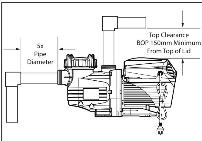
Figure 7. Viron XT Series 2 Pump Piping Clearance
