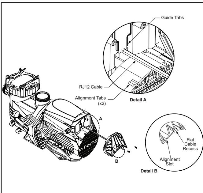
Figure 10. Data Port Location on XT Pump
