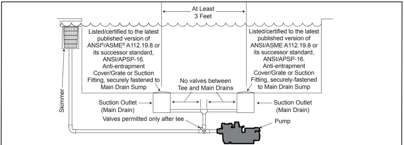
Figure 9. Number of Suction Outlets Per Pump
