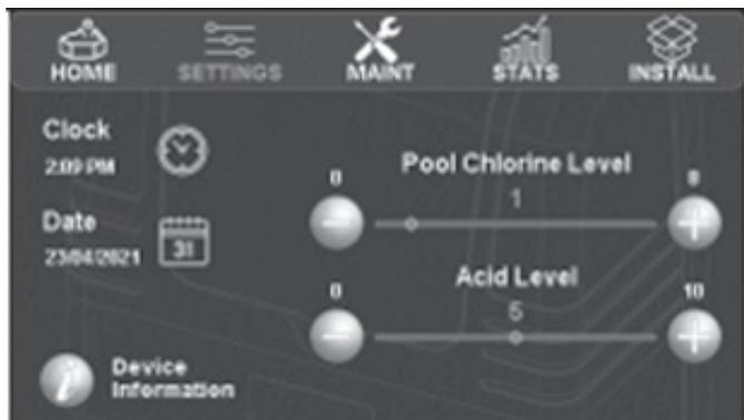
Figure 34. Halo Pool Chlorine and Acid Level Screen
