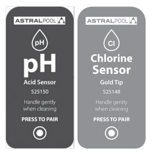
If a pH sensor and an acid dosing pump have been configured (See acid dosing pump instructions), then a Gold Chlorine ORP sensor can also be paired to the Halo Chlorinator using the "Add/Remove" button and choosing "ORP Sensor".
