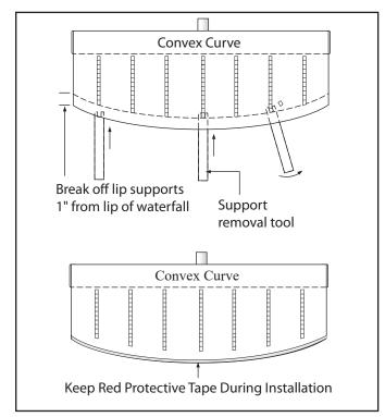
Figure 17. Custom Waterfall Installation - Convex Curve
