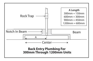
Figure 5. Plumbing for 300mm through 1200mm Lengths
