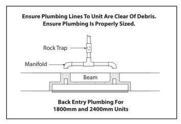
Figure 13. Single Waterfall Plumbing for 1800mm and 2400mm
