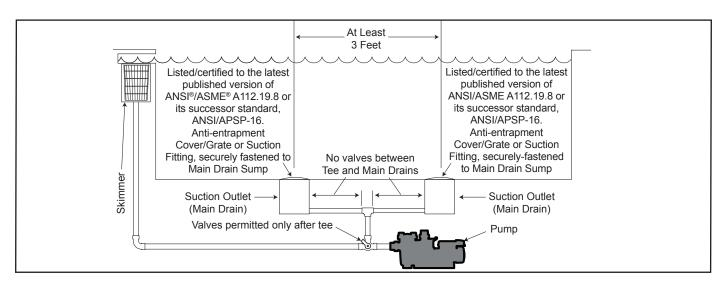
Figure 1. Number of Suction Outlets Per Pump
