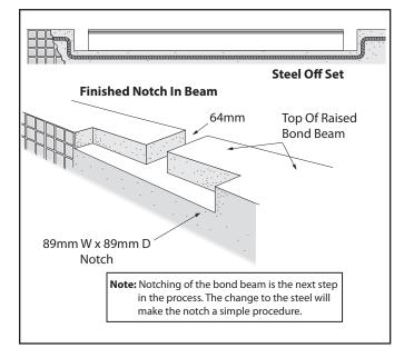
Figure 3. Excavation and Steel Installation
