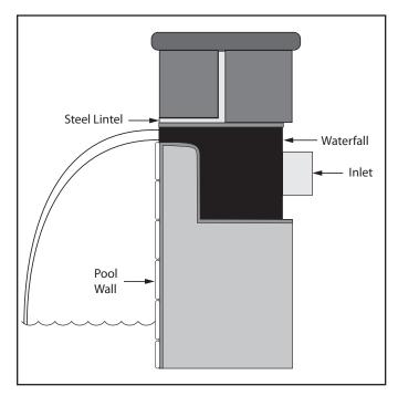
Figure 7. Lintel Installation for 1" Lip Back Entry Waterfall
