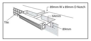
Figure 4. Concrete Installation
