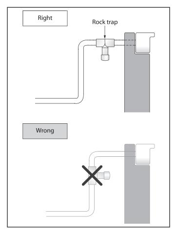
Figure 21. Rock Trap Debris Chamber Installation
