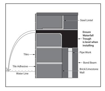
Figure 8. Lintel Installation for 6" Lip Bottom Entry Waterfall
