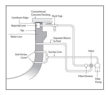
Figure 10. Filter Pump Installation
