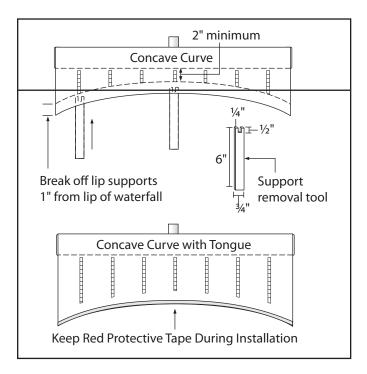
Figure 18. Custom Waterfall Installation - Concave Curve
