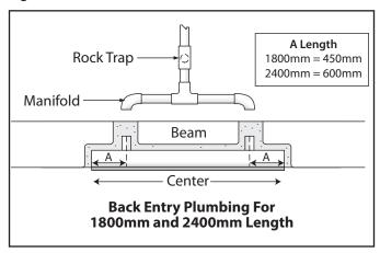
Figure 6. Plumbing for 1800mm and 2400mm Lengths
