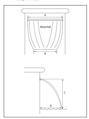
Figure 9. Waterfall Measurements for 300mm to 2400mm Models
