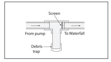
Figure 20. Rock Trap Installation
