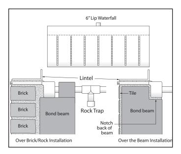
Figure 16. Extended Lip Waterfall Installation
