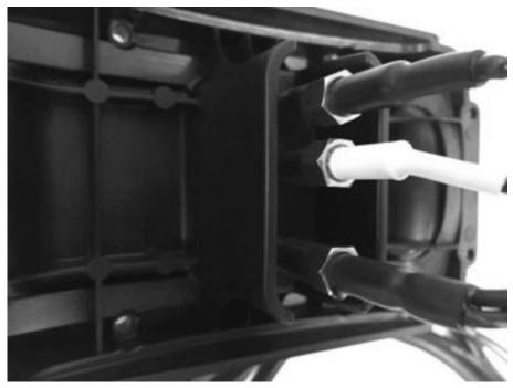
Tighten the nuts with a suitable spanner to secure the cell connectors to the titanium rods, on the EMX3600 once applied. Hold the back of the cell leads when tightening.
