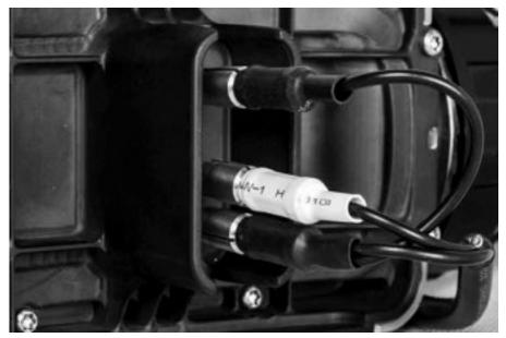
Tighten the "push on cell connectors" on the EMX2400 by using a pair of pliers, once applied.
