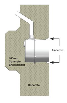
Diagram 1 - After Concreting
