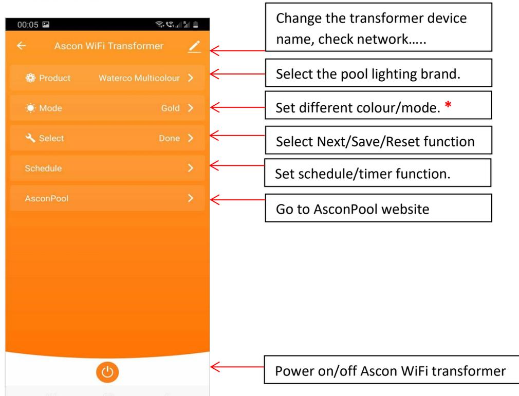
**\* Colour modes for multiple pool lights are in the MODE menu. If a colour is chosen that IS NOT part of the sequence for your light, the TXF will not change.**
