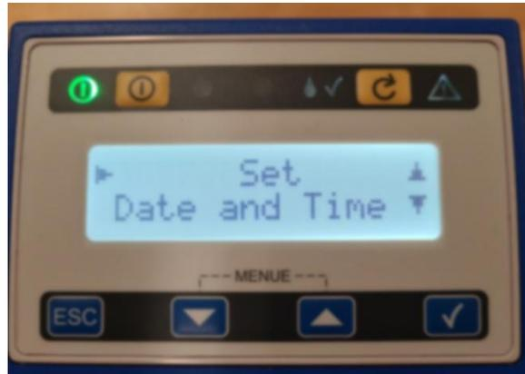
Once in the setting, change the date and time to the current Australian Eastern Standard Time (AEST). To scroll through the setting in each menu use the tick button (✓) to scroll right and the ESC button (ESC) to scroll left. Use the up and down button to change the setting values. When completing any changes in the menu always click the tick button to get to the end of the changes to save the settings.
