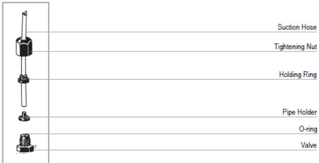
**Figure 5.11 Connection Point Assembly6**
