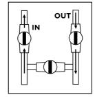
When your valves position are as shown on Figure 2, the water is going through the pool heat pump.
