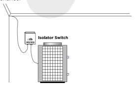
A WARNING THE POOL HEAT PUMP MUST BE DISCONNECTED BEFORE OPENING THE ACCESS PANEL.
