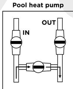
When your valves position are as shown on Figure 1, the water is bypassing the pool heat pump.
