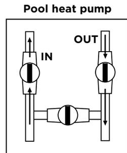
When your valves position are as shown on Figure 2, the water is going through the pool heat pump.
