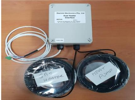
The Kit 13 Dual Heater Interface (8519128) is designed to be connected to the Pooltek unit and switch between 2 heating sources (Gas Heater & Heat Pump) where the Heat Pump is utilised for heating the pool and the Gas Heater is utilised for heating the spa. The Gas Heater can also be over-riden to heat the pool.
