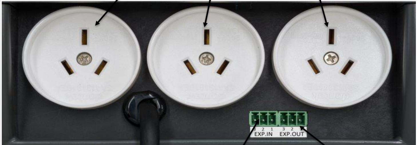
If Expansion Unit 1, the connection cable from the master controller will plug in here. If Expansion Unit 2, the connection cable runs from here to Expansion unit 1 EXP OUT.
