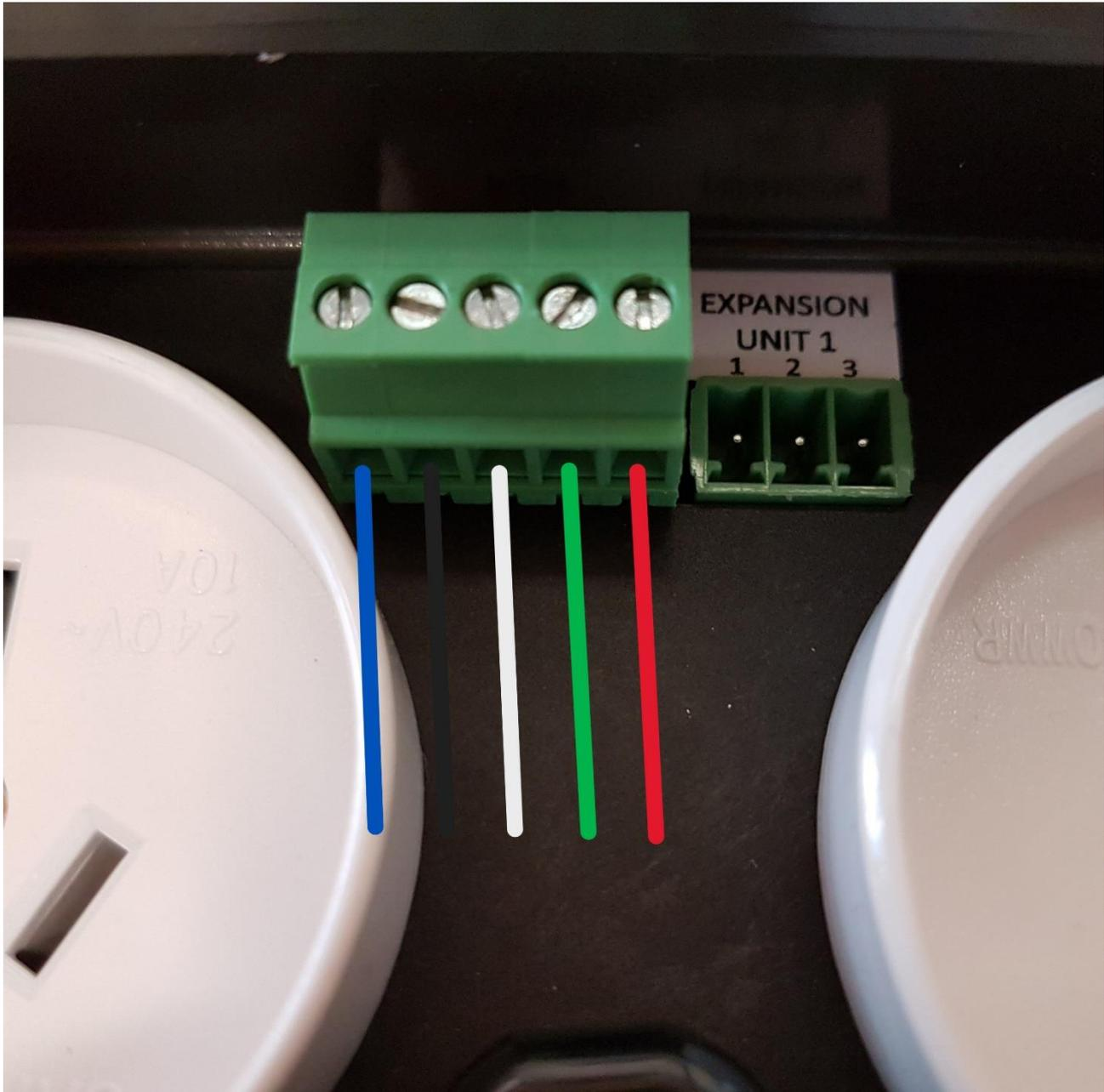
**WATERCO ECO-V VARIABLE SPEED PUMPS MAY BE CONTROLLED VIA THE POOLTEK SPEED CONTROL FUNCTION BY INSERTING THE CONTROL CABLE WIRES INTO THE PUMP CONTROL TERMINAL BLOCK. THE WATERCO PUMP CONTROL CABLE SHOULD BE USED AND THE PLUG SOCKET REMOVED TO ALLOW WIRE TERMINATION INTO THE FIVE WAY SCREW TERMINAL AS PER THE ABOVE PICTURE.**
