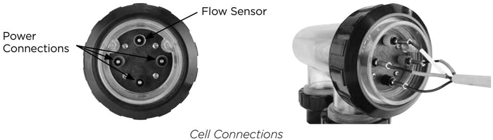
Ensure that the 4 connections (3 for cell power and 1 for flow detection) are not loose. A loose connection is likely to cause arcing, which may damage the entire system.
