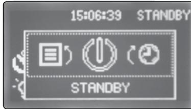
When selecting STANDBY, Electrochlor switches the pool pump off and disregards current timer cycle programming. The Electrochlor will resume normal programming functions with the next timer cycle if AUTO or WINTER modes are active.
