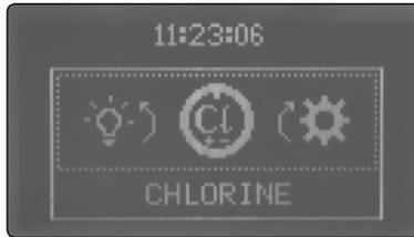
Rotate the wheel to the right to raise production. If the pool water is over chlorinated, simply reduce the chlorine production set level by rotating the wheel to the left. Press the wheel confirm the desire chlorine output.
