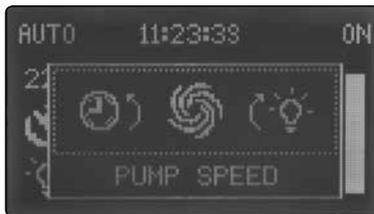
Use the wheel to select the desire pump speed. Rotate the wheel to check mark (✓) and press to confirm or select X to exit without saving.
