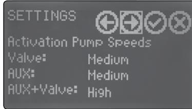
If the minimum speed is not reached during the Interlock functionality, interlock is disabled. This also puts a restriction defining the pump speed in the timer. If the minimum speed does not fulfill the pre-set requirements, Electrochlor won't allow the interlocking function. This is to ensure that the minimum water flow is provided for the ancillary function to operate.
