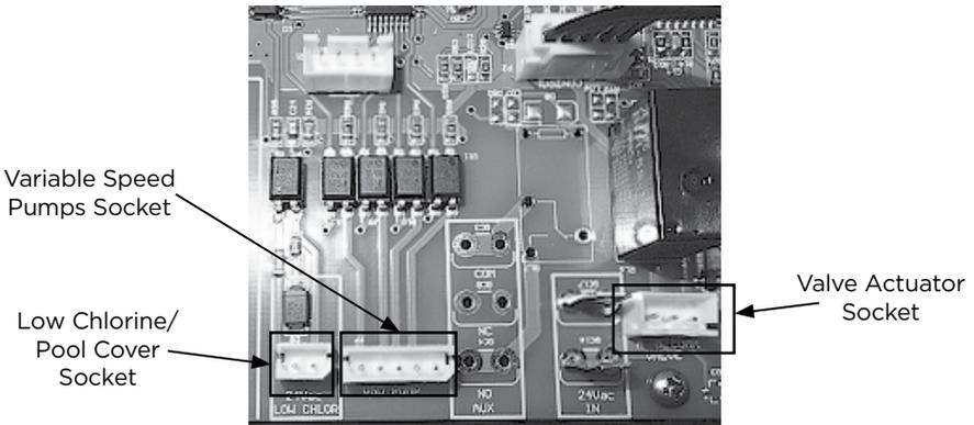
*Main Board showing ECO Pumps Socket, Valve Actuator and Low Chlorine/Pool cover connections.*
