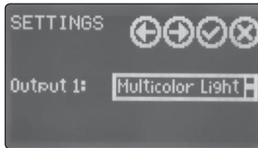
iii. Changing Light colour: navigate in Setting to light colour, rotate the wheel to select the colour. This is only compatible with Waterco's multicolour lights.
