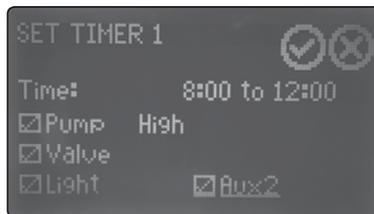
Figure showing Interlocked functions programmed through timer meeting the minimum pump required speed, in this case high.
