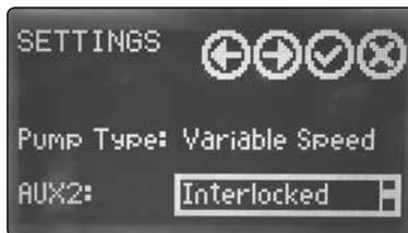
2. Define actuation speed: Access setting menu and select the minimum allowed pump speed that enables the interlocked functions:
