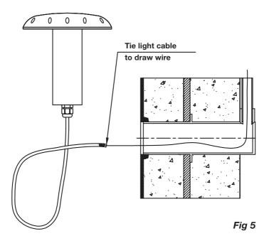
Before pulling all of the 20m power cable through the electrical conduit and fixing the LED into the niche, the LED light needs to be prepared for permanent installation into the niche using PVC glue.
