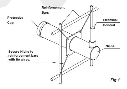
Make sure the niche socket and conduit connection is not covered by concrete during the forming process. refer to fig 2.
