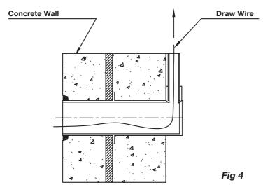
If not previously done, at this stage it would be recommended that a draw string be passed through the niche and electrical conduit to aid in the installation of the actual light and electrical cable.
