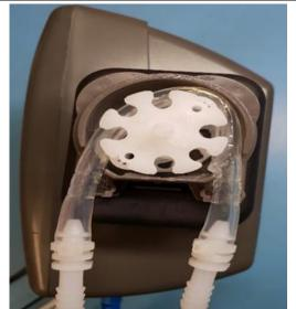
The pump head can be pulled out (the squeeze tube will come with it) and a new squeeze tube can be wrapped around the head, and the head re-installed onto the motor shaft.
