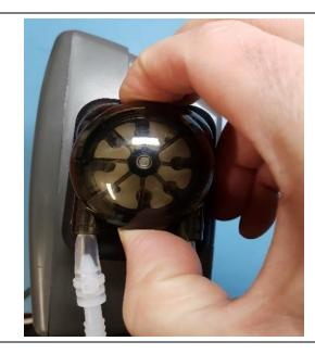
The head cover will come off to expose the squeeze tube and the head.
