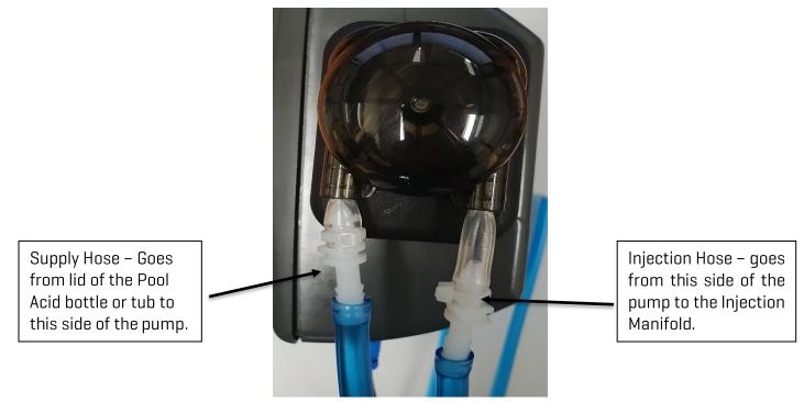
HINT: -Soak the ends of supply and injection hoses in hot water for 30 seconds to soften them, this will make it easier when fitting the tubes to the pump barbs.
