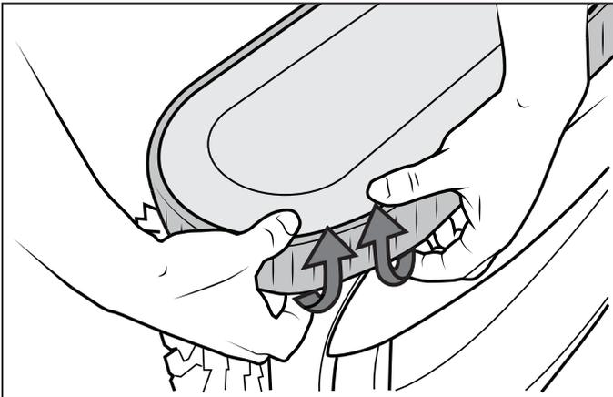
Figure 28. Pull the Old Track Over the Wheel
