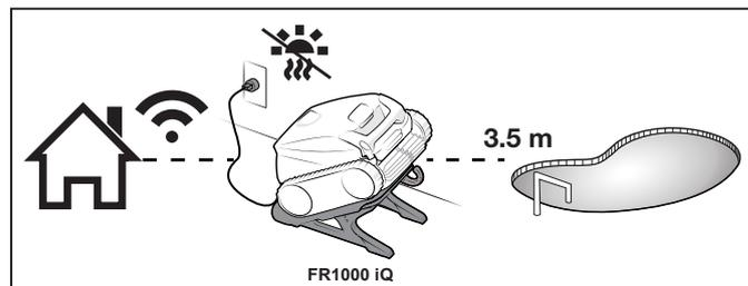
Figure 17. Charging Station Distance to Pool Edge
