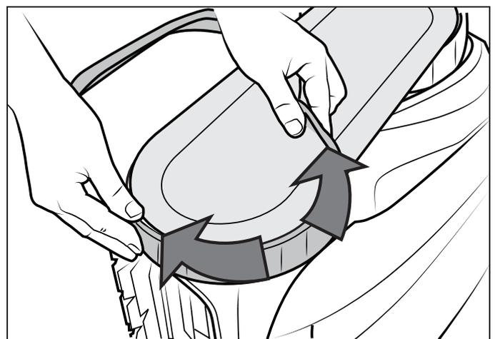
Figure 32. Work the Track On Around the Wheel
