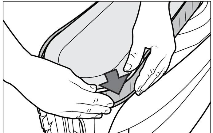
Figure 31. Start on One Side of the Track
