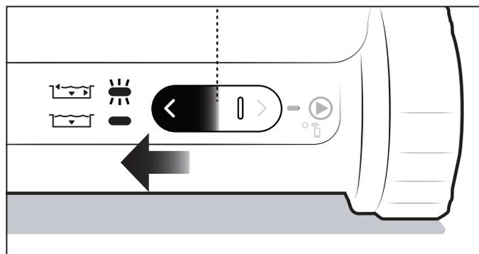
**Figure 7. Slide and Release Left to Select Mode**
