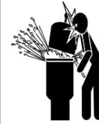
THIS FILTER OPERATES UNDER HIGH PRESSURE. WHEN ANY PART OF THE CIRCULATING SYSTEM (e.g., FILTER LID, PUMP, FILTER, VALVES, ETC.) IS SERVICED, AIR CAN ENTER THE SYSTEM AND BECOME PRESSURIZED. PRESSURIZED AIR CAN CAUSE THE LID TO BLOW OFF WHICH CAN RESULT IN SEVERE INJURY, DEATH, OR PROPERTY DAMAGE. TO AVOID THIS POTENTIAL HAZARD, FOLLOW THESE INSTRUCTIONS.
