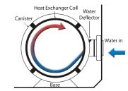
✓ Powerful heat transfer through the dual coil heat exchanger maximising water contact
