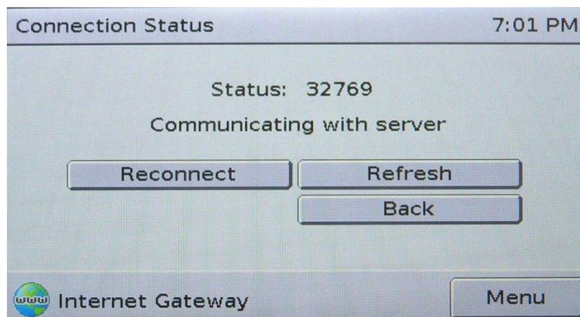
If the status is shown as '?', then the Touchscreen cannot communicate with the Internet Gateway. Check that the Internet Gateway is plugged in to the pool system, using normal flat-cable RJ12 connection, and that the plugs of the RJ12 cable have the correct orientation.
