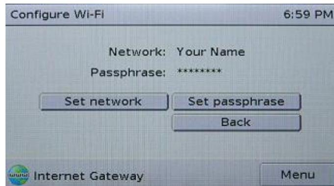
5. From this screen, press 'Set network'. Use the Backspace button to remove the 'Your Name' text and then use the keyboard to enter the name of your home Wi-Fi connection. Similarly use the 'Set passphrase' key to set the passphrase/password of your home Wi-Fi connection. **Network names and Passphrases are case sensitive- make sure you enter them correctly and exactly otherwise system will not connect to network.**
