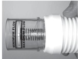
Switch the pump on and start adjusting the Knob of the Regulator Valve "Faster" or "Slower" until the disc indicator in the Flow Gauge settles between "maximum" and "minimum" flow.
