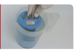
There will be a reaction as the calcium is dissolved. When the reaction ceases (about 10 minutes) rinse the electrode in clean water, wipe the brass terminals dry and check that all calcium has been dissolved. If not, repeat the process with a new solution.
