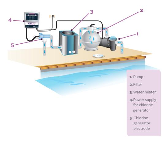
The SMC chlorine generator can be fitted to pools with any type of heating system. Do not install chlorine generator and water heater in reverse as the heavily chlorinated water could damage the heating unit and may negate the heater warranty.
