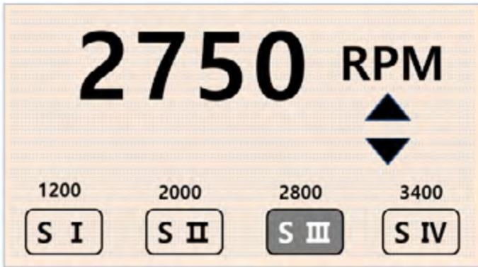
Select the Button that represents the Speed you wish to adjust. Once selected the speed will appear at the top of the screen, then press the “up” or “down” buttons to select the speed you want, changes are in 25 rpm increments. Once speed is selected this will be automatically saved. Continue this process to change the speeds are you require.
