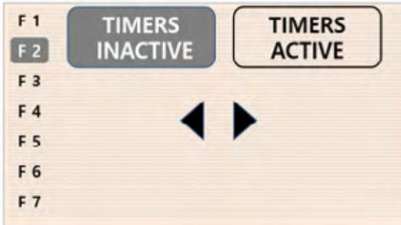
If “Timers Active” selected, screen will then displays timer 1 (T1) to Timer 4 (T4) above 4 horizontal buttons beneath LCD screen and a summary of timer periods as below.
