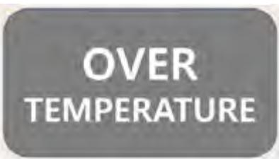
Your Insrng Variable Speed Pump has capability of measuring the Temperature of the Motor and outside conditions. Should temperature reach above standard operating levels, the pump will stop until temperature drops and the below will display on the screen.
