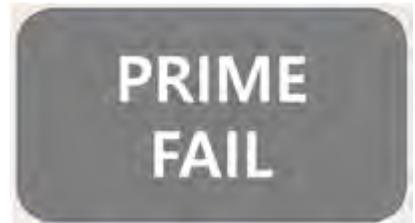
Pump Motors require additional current at start-up to get running. Should the above display, the Pump has not been able to get enough current to operate on start-up. This could be due to too many electrical items on the one connection draining current from the Pump, or due to change in your local supply. Suggest removing any unnecessary items and restart. If still shows display warning, contact your local pool professional for assistance.
