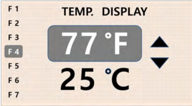
Press up or down to select your preferred display in either “C” (Celcius) or “F” (Fahrenheit). If no external temperature sensor is fitted to your Pump the display will show “0” values, contact your pool professional to confirm if this is correct.
