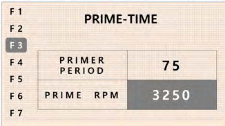
When “on” is selected “primer period = mmm: XXX”. Press up or down to select from “0” to “120” minutes. Scroll right or left to select Prime RPM, press up or down to select 1200 to 3300 in 25 RPM increments.
