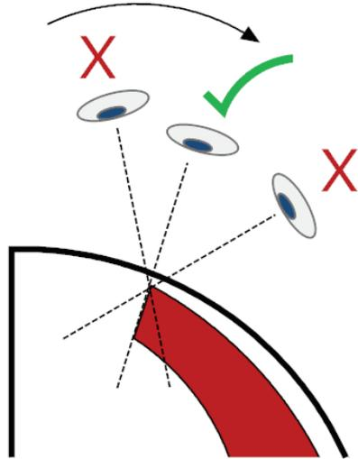
**NOTE:** *Slowly move your head in this direction to the point where the leading edge of the indicating arm is not visible.*
