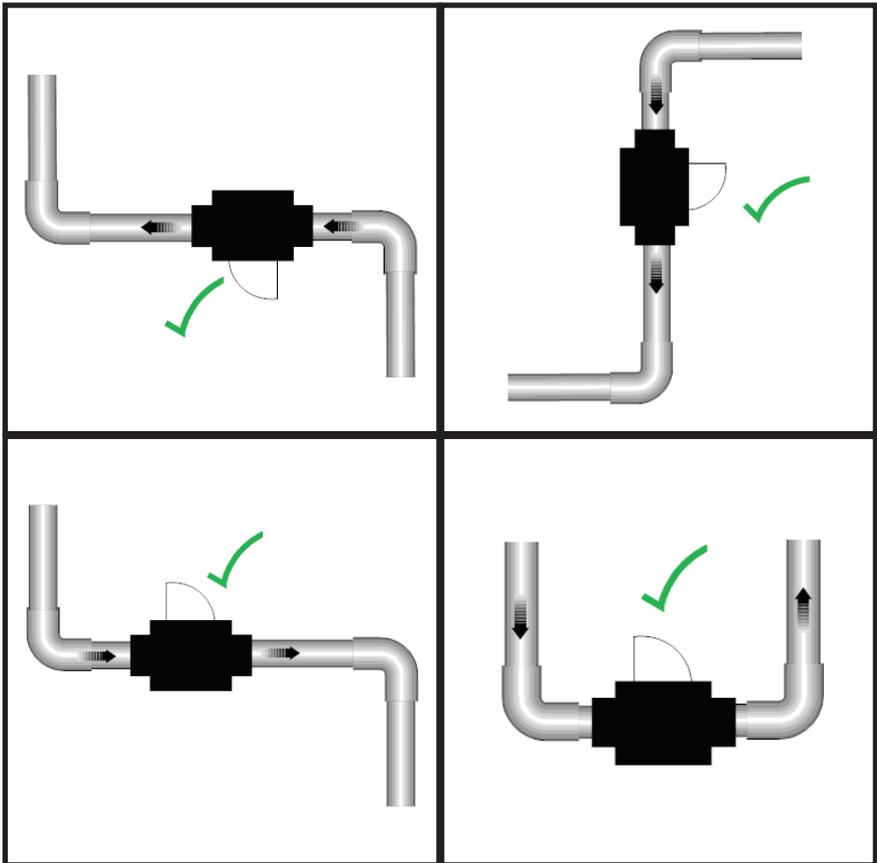
**NOTE:** When selecting a physical location to install FlowVis®, be sure to allow accessibility to read the scale on the lid.
